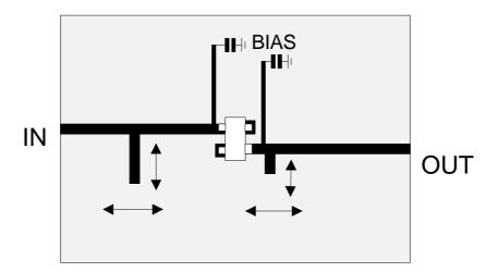
On this universal printed circuit board it is possible to match all (!) impedances to  $50\Omega$  by applying movable open stubs with about  $50\Omega$  impedance and variable length. The stubs can be realized by copper or brass foil which can be moved by the soldering iron and cut in length. If it is too short it can be replaced by a new one. The method is a simple cut and try strategy but very fast and effective.
