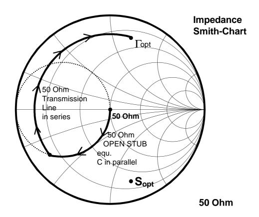
An example in the smith chart shows, that all needed impedances can be realized on the universal printed circuit board.
