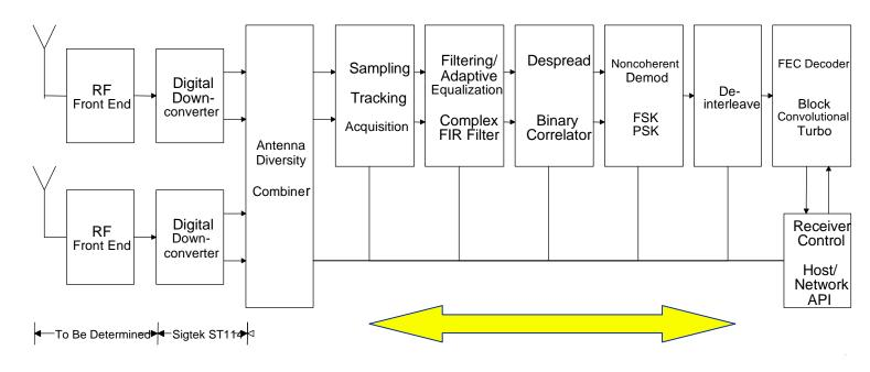
Direction for replacement of DSP  $\mu$ P functions with reconfigurable computing
