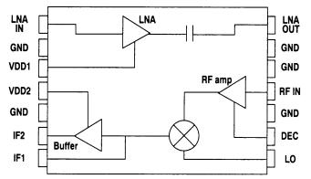
3. This LNA/Mixer IC is optimized for minimum current drain at +3 VDC.
