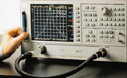
Productivity is enhanced with pass/fail testing, direct printer/ plotter output of results, advanced marker functions, save/ recall of test configurations to internal memory or a built-in floppy disk drive, and test sequencing for automation. Options allow high-power tests, frequency offset mixer testing, and high-accuracy noncoaxial and on-wafer measurements.
