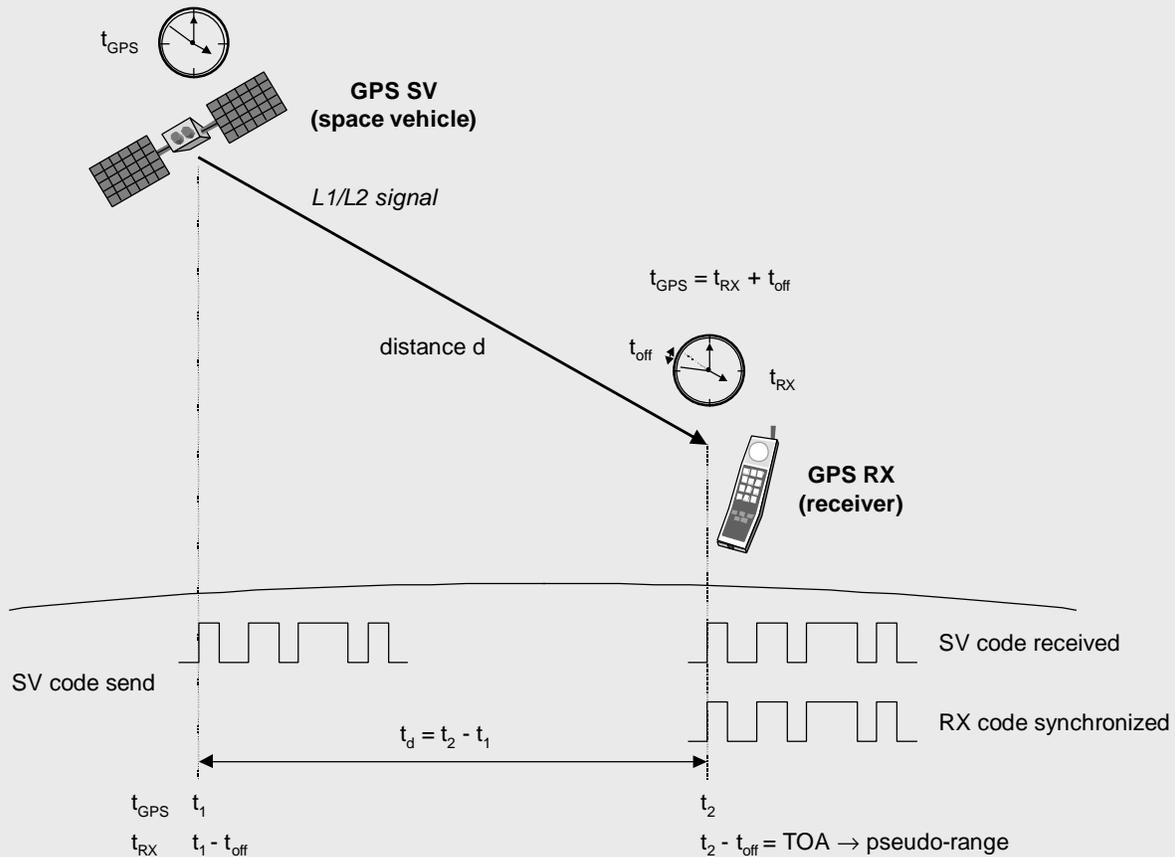
If the receiver clock is perfect, than all the satellite (SV) ranges would intersect at a single point (which is the position of the receiver). Three perfect measurements can locate a point in 3-dimensional space.
