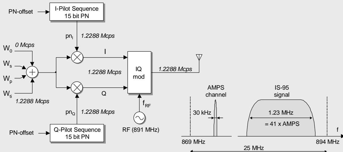
The bandwidth of a CDMA signal is 1.23 MHz. The bandwidth of an AMPS channel (using the same frequency band) is 30 kHz. Therefore the bandwidth of a CDMA signal corresponds to an aggregate bandwidth of 41 AMPS channels.
