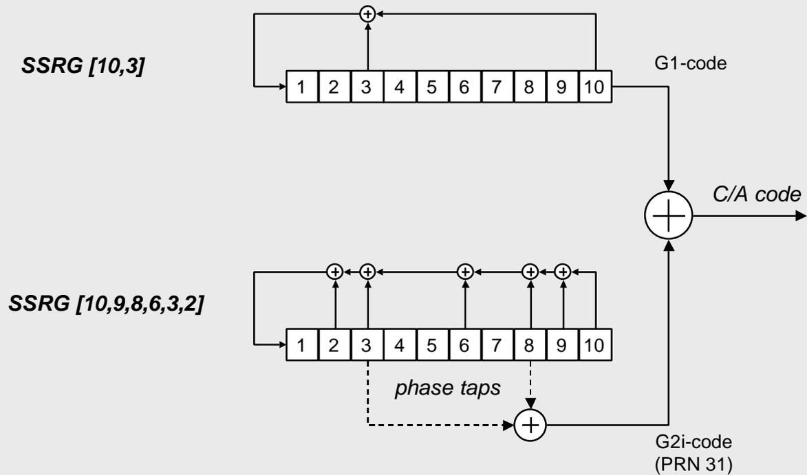
The C/A code generator produces a different 1023 chip sequence for each phase tap setting.
