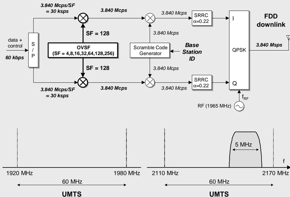
Traffic data (voice) is multiplexed with control information (pilot bits, transmit power control bits, rate information, ...). The serial-to-parallel converter maps the 60 kbps to the I and Q branch of the QPSK modulator. This produces a 30 ksps symbol rate. The I and Q branches are then spread to the 3.840 Mcps chip rate with the same Orthogonal Variable Spreading Factor (OVSF) code. Since the spreaded bandwidth is the same for all users, multiple-rate transmission needs
