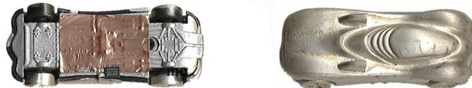
**FIGURE 3.3.7** A TouchTag enabled toy car with an RFID tag chip. It could still function if coated with a nonconducting outer surface.
