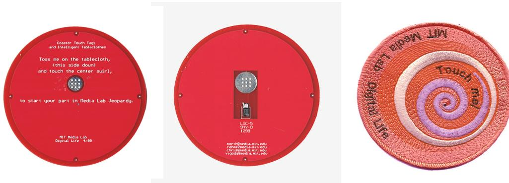
**FIGURE 3.3.6** TouchTags used as tabletop login tokens for “Tablecloth Jeopardy Game” TTT Spring 1999. Views from left to right: Bottom, Top (with Swatch RFID tag chip), and “Ebroiderery [POS97]” Top Cover.
