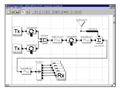
UNIstar models a radio system with a set of circuits composed of interconnected equipment. A group of related circuits is called a system configuration, or just configuration. A block diagram is used to depict each of the individual circuits in a configuration. These circuits define the equipment used and the current path from an antenna to a transmitter or receiver.
