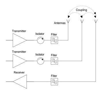
Passive intermodulation can be reduced by minimizing the number of loose metallic joints<sup>2</sup> within system components such as antennas, cables and connectors, and in the external environment on towers and wire fences.
